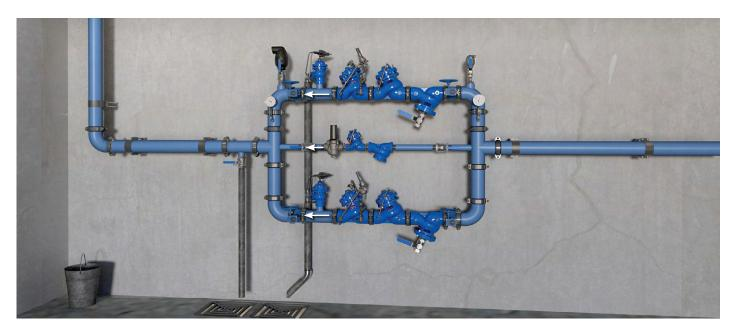
**Two-Stage Pressure Reducing Station**, featuring BERMAD BC-720-PD-P valves to reduce the incoming pressure by a fixed ratio and share the load with the BERMAD BC-720-P PRV, a redundant, parallel branch to minimize the possibility of total water shut-off and a low flow
