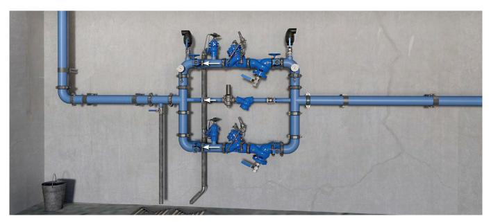
Pressure Reducing Station, featuring BERMAD BC-73Q-P valves to relieve excessive downstream pressure, a redundant, parallel branch to minimize the possibility of total water shut-off and a low flow bypass branch for low demand operation. For information on the other BERMAD products in this system please see the product data sheet for the BERMAD BC-720-P and BERMAD BC-70F-P.
