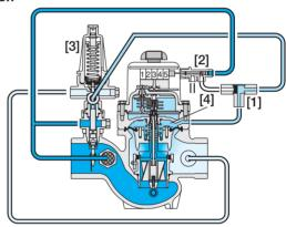
The Shuttle Valve [1] hydraulically connects the Shut-Off Pilot (SOP) [2] or the Paddle Flow Pilot (PFP) [3] to the AMV Control Chamber [4]. The PFP commands the AMV to throttle closed should demand rise above setting, and to modulate open when demand drops below setting. Upon delivering the preset quantity of water, the SOP switches and pressurizes the shuttle valve, which thereby transmits this pressure into the control chamber, causing the AMV to shut.
