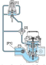
The Hydrometer continuously transmits flow data to the irrigation controller. The Pressure Sustaining Pilot [1] commands the Hydrometer to throttle closed when Upstream Pressure [P1] drops below setting, and to open fully when [P1] rises above pilot setting.
