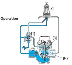
The 3-Way Hydraulic Relay Valve (3W-HRV) [1] hydraulically connects the Pressure Reducing Pilot (PRP) [2] to the Hydrometer Control Chamber [3]. The PRP commands the Hydrometer to throttle closed should Downstream Pressure [P2] rise above setting, and to open fully when it drops below setting. The 3W-HRV switches upon pressure drop command, directing line pressure into the control chamber, and thereby causing the Hydrometer to shut. The 3W-HRV also features local manual closing.
