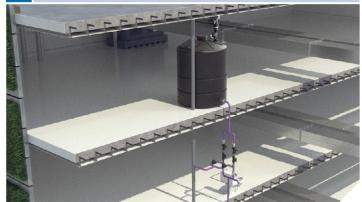
Teated Recycled water for sanitation use - using cooling towers water for toilet flushing, floors washing and irrigation.
