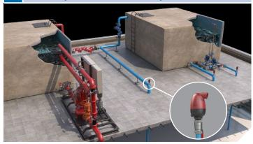
Roof-top Potable Water and Fire Protection reservoirs, Level Control with Backup and Overflow Protection systems, Pumps Station for upper floors boost, Pressure Relief valves.
