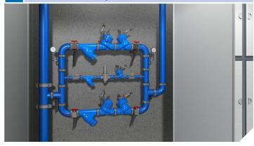
Potable Water Multi Zone Supply PRV Station with redundancy back-up branch and secured excessive pressure emergency valve – High pressure protection with no water discharge.
