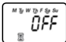
The irrigation duration value displays OFF or the previously programmed duration of irrigation. Please note that the word OFF appears when the duration of irrigation is set to zero.
